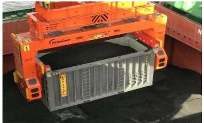
*Image: Sealed rotainers would be loaded from within the portside shed, and onto trailers, and driven to the wharf. The rotainers would be lowered into the hull of the vessel, rotated and the product discharged*
