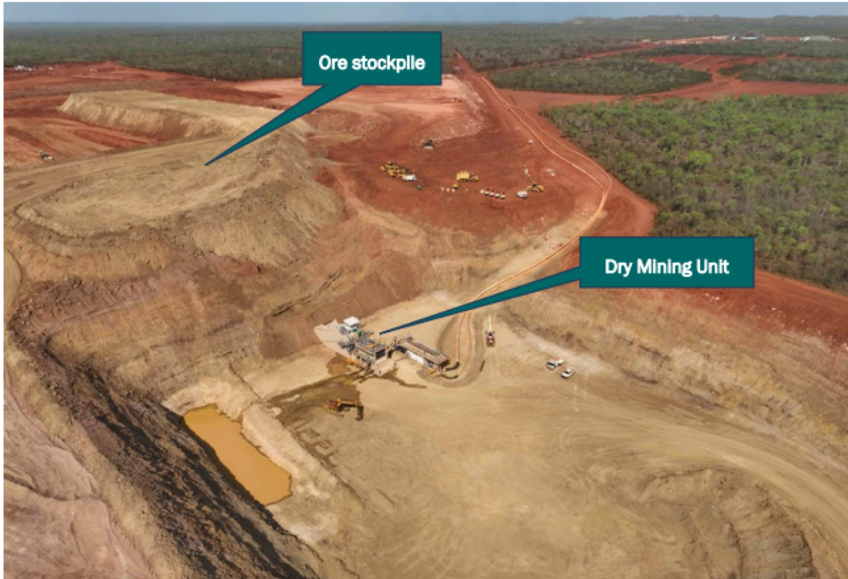
Image: Mining area with ore stockpile and Dry Mining Unit
